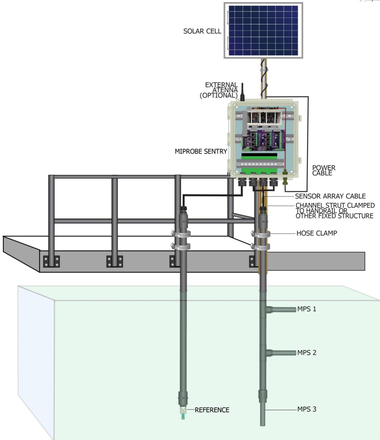
Figure 14: Vertical Sensor Array Configuration
