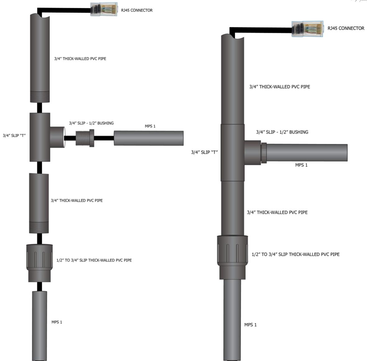
Figure 11: Multiple MPS Mounting System
