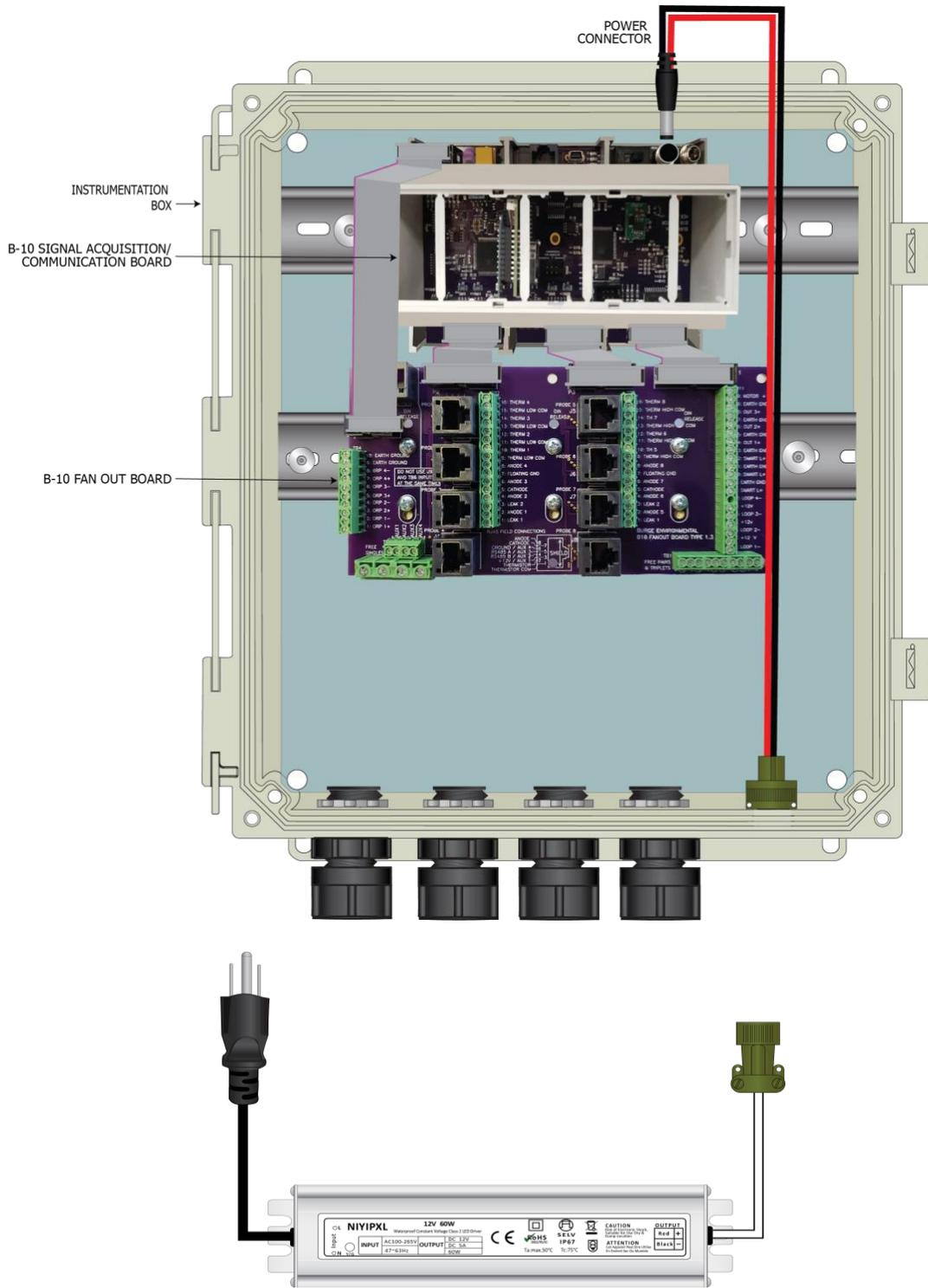
Figure 7B: 12-Volt Power Supply Option: Series 200
