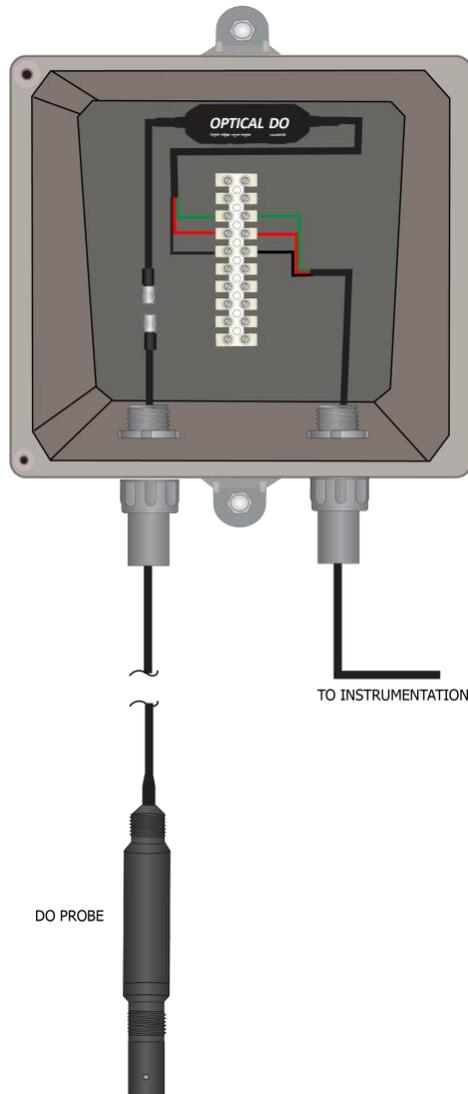
Figure 27: Mounting of Auxiliary Sensors: Auxiliary Box
