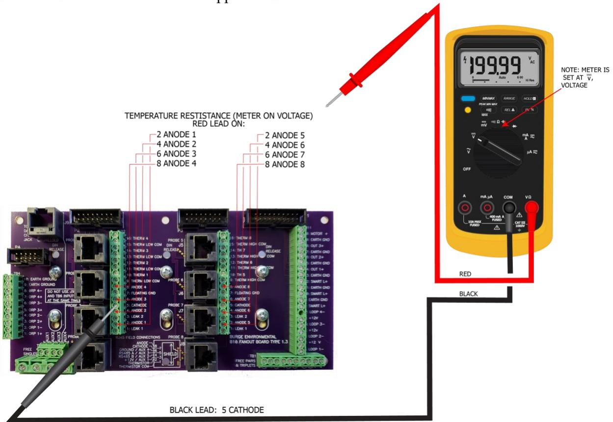
Figure 34: Measurement of Microbial Sensor: Voltage
