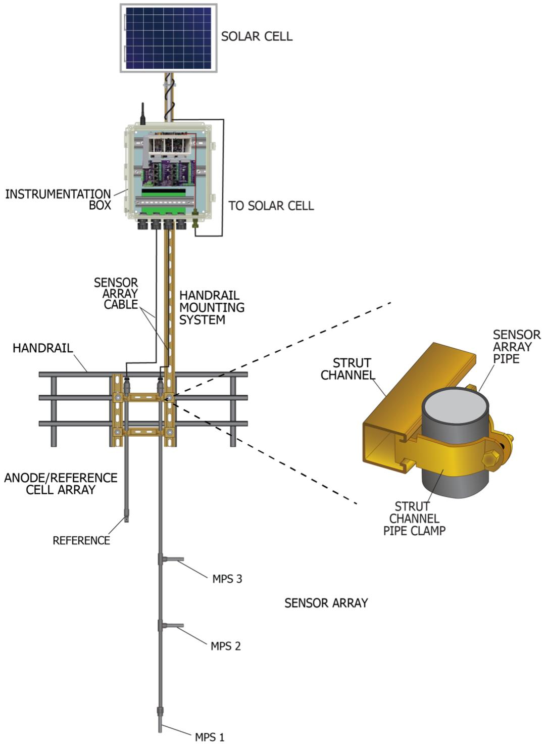
Figure 23: Mounting of Sensor and Reference Cell Arrays to the Handrail Mounting System
