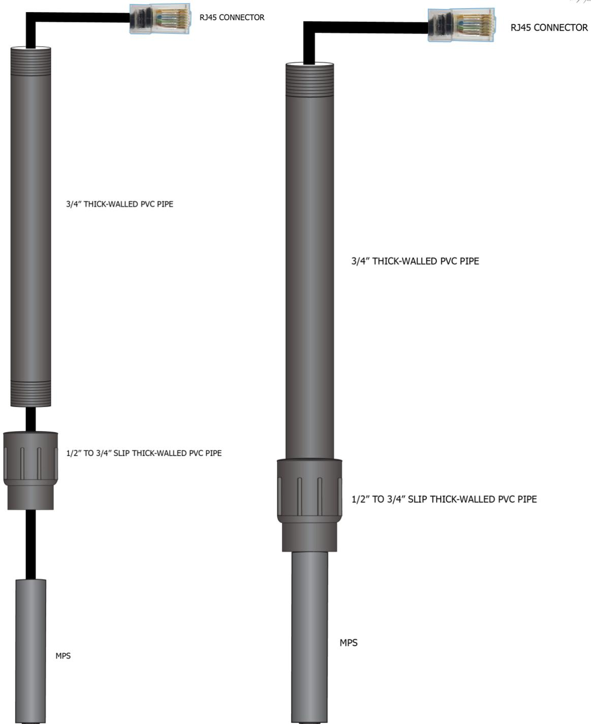
Figure 10: Single MPS Mounting System
