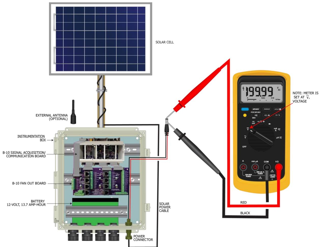
Figure 33A: Measurement of the voltage from the solar cell
