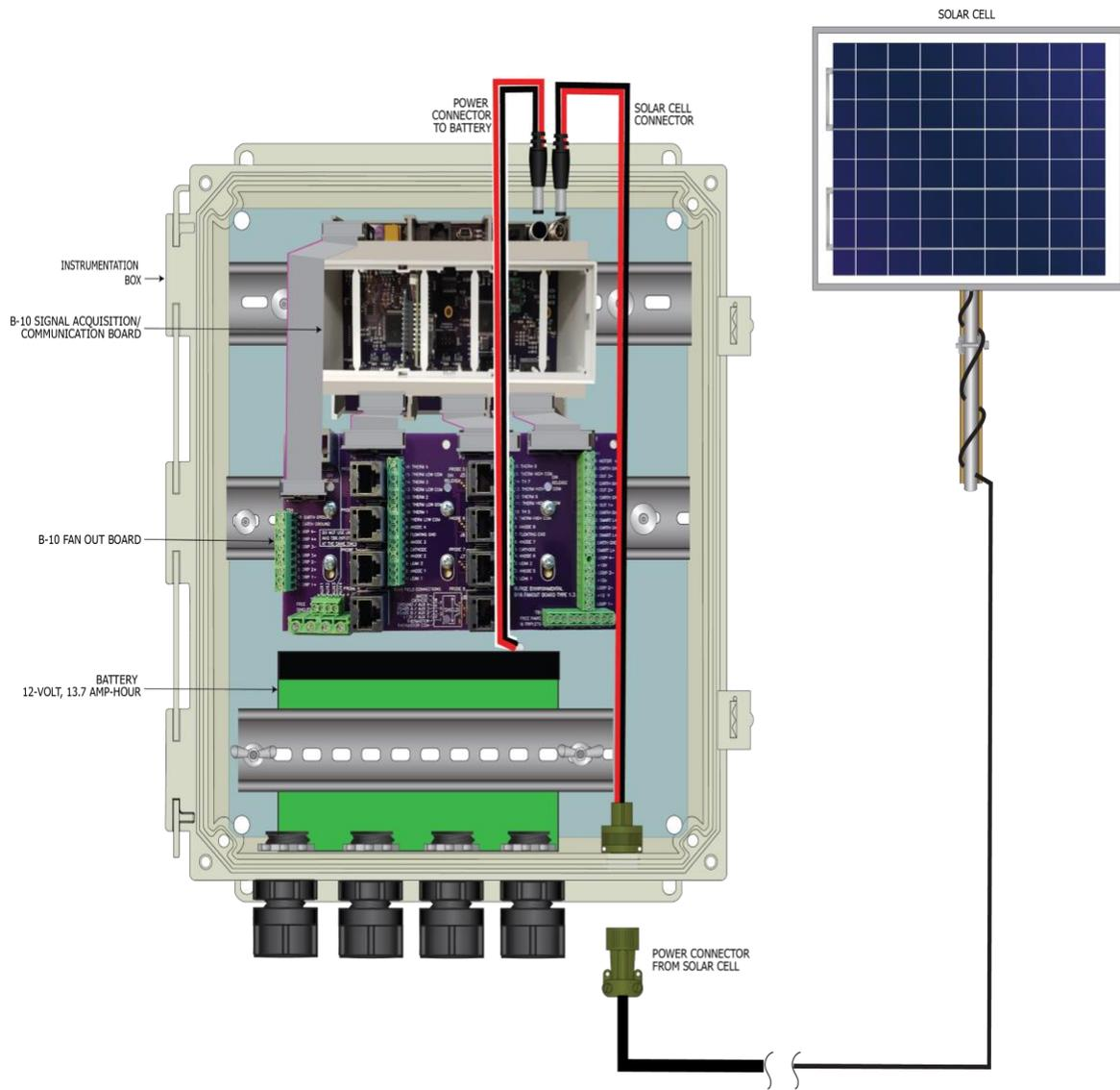
Figure 7A: Solar Cell/Battery Power Option (Series 100)
