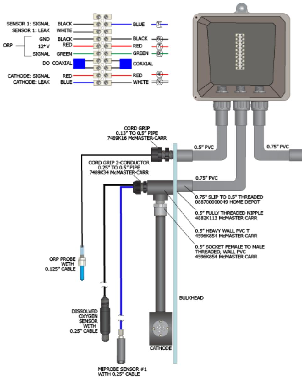
Figure 31: Auxiliary Box for Microbial Sensor, Cathode and Auxiliary Sensors
