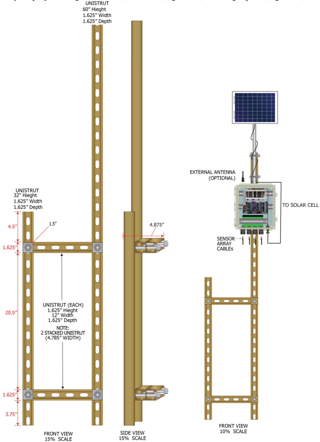
Figure 19: Handrail Mounting System
