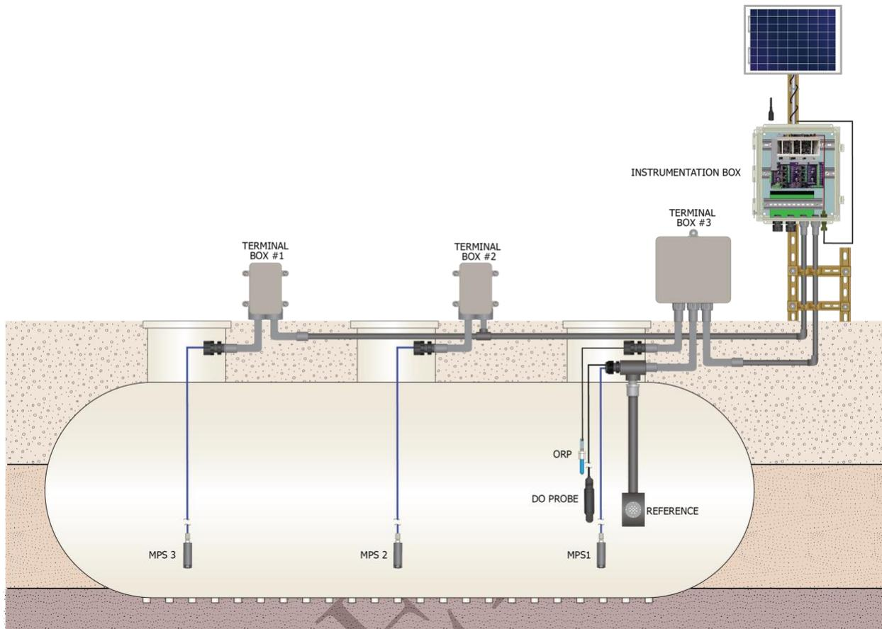
Figure 16: Horizontal Sensor Array Configuration
