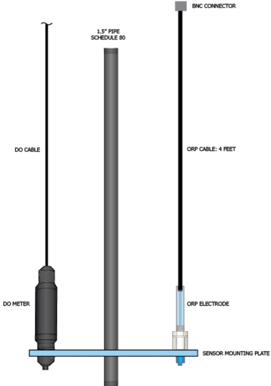
Figure 18: Auxiliary Sensor
