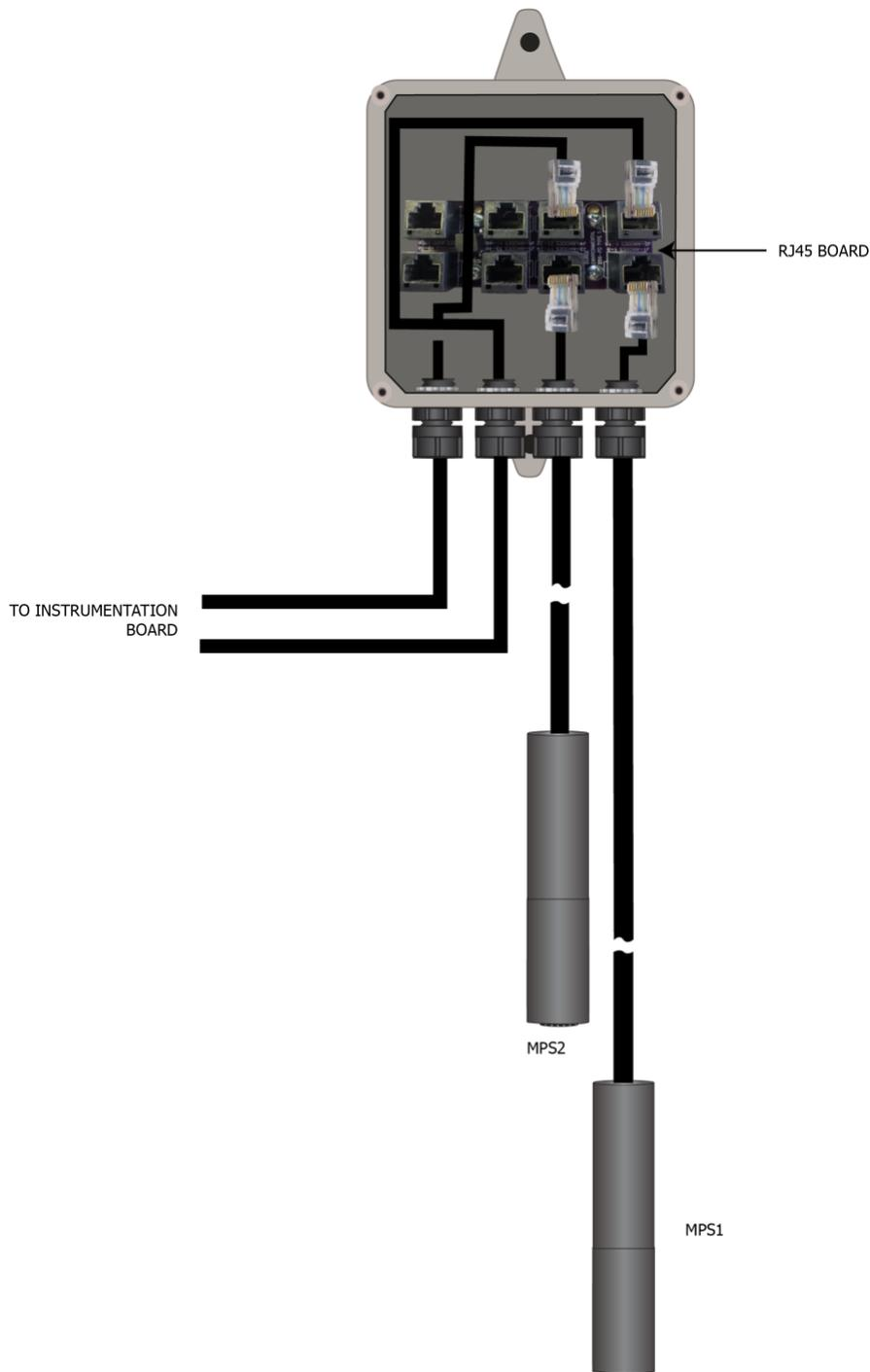
Figure 28: Auxiliary Box and MPS sensor termination (JP-45).
