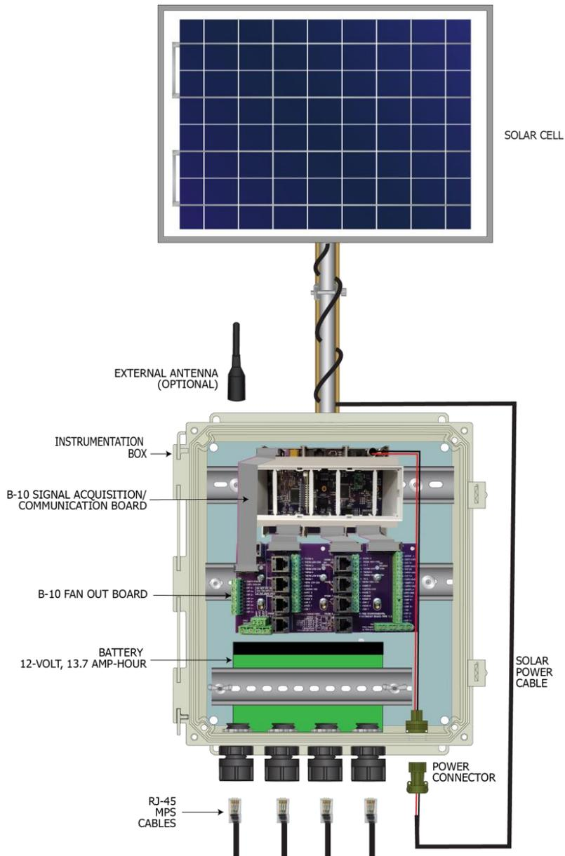
Figure 25: Instrumentation Box (Series 100): Solar Power Configuration
