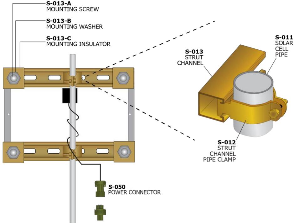
Figure 22: Mounting of the Solar Cell Assembly
