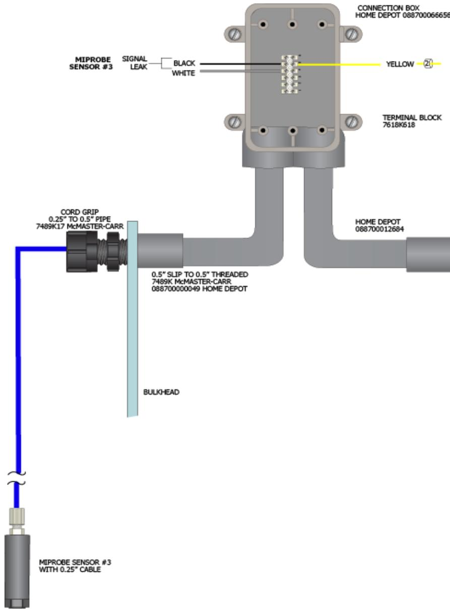
Figure 29: Auxiliary Box with terminal block for Single Microbial Sensor: Subsurface Horizontal Deployment
