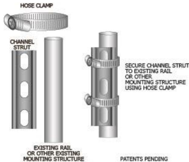
Figure 20: Single-Pole Mounting System
