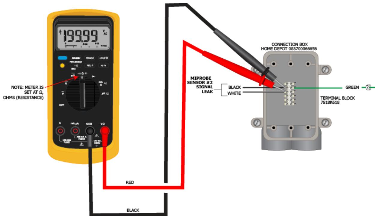
Figure 36: Measurement of Microbial Sensor Leaks: Resistance
