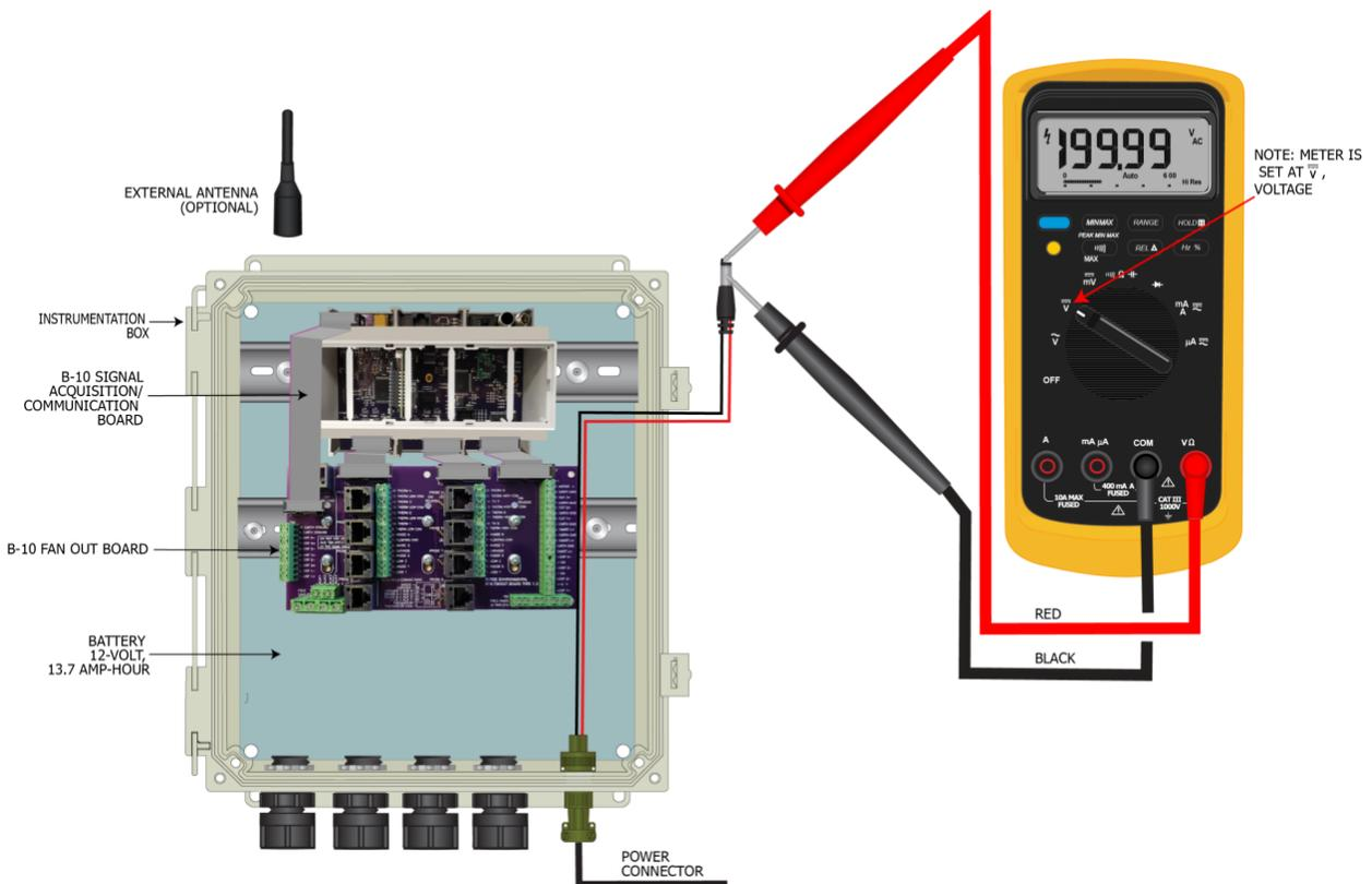
Figure 33C: Measurement of the voltage from 12-volt power supply
