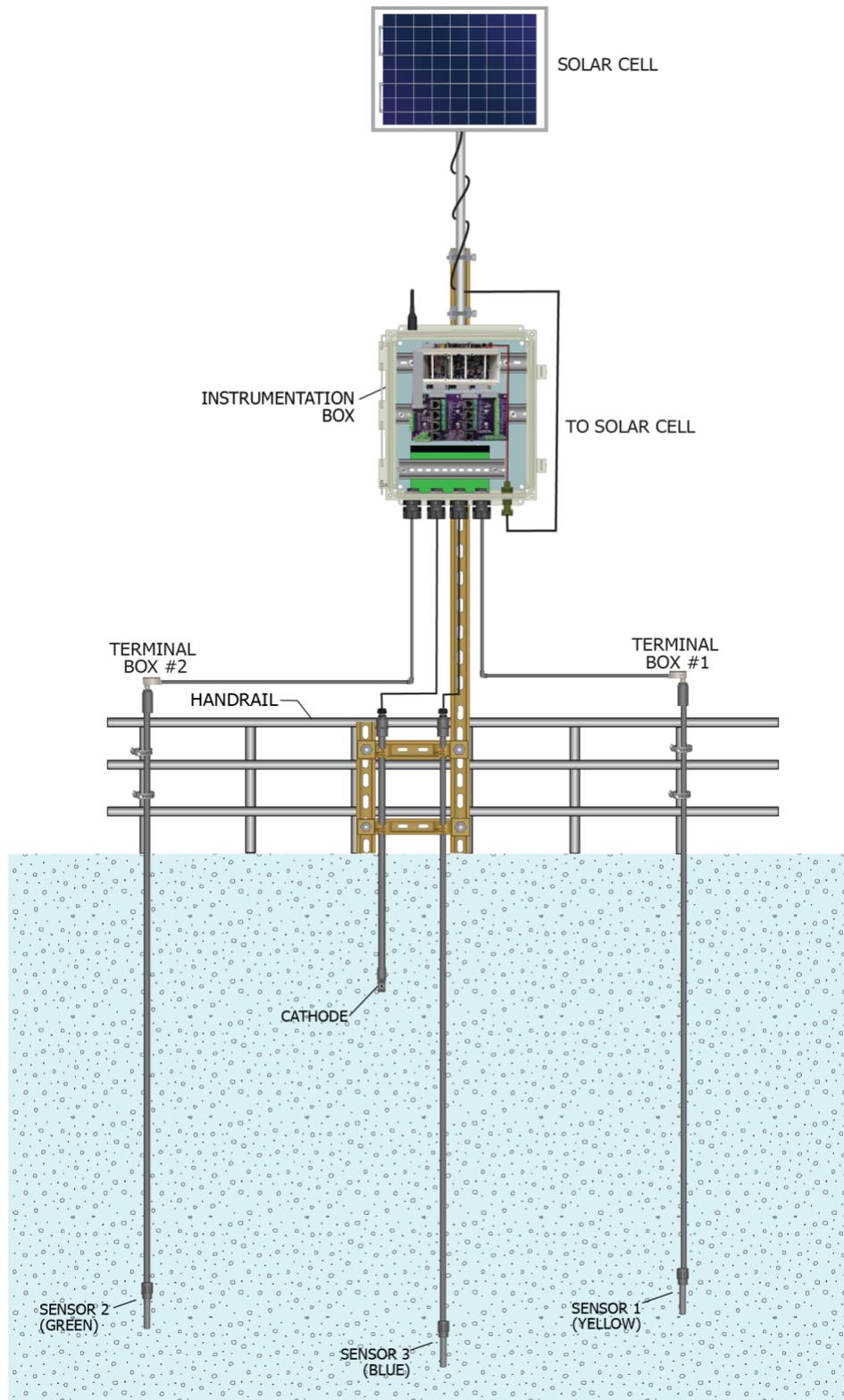
Figure 32: Microbial Monitoring System: Horizontally-Distribution System located Above Ground Surface
