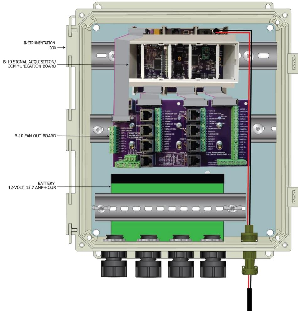
Figure 2: MiProbe Instrumentation Box: Series 100
