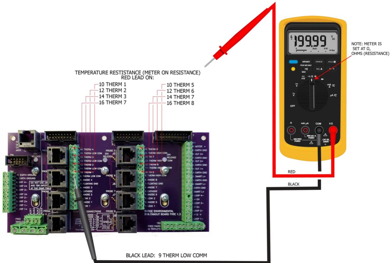
Figure 35: Measurement of Thermistors: Resistance
