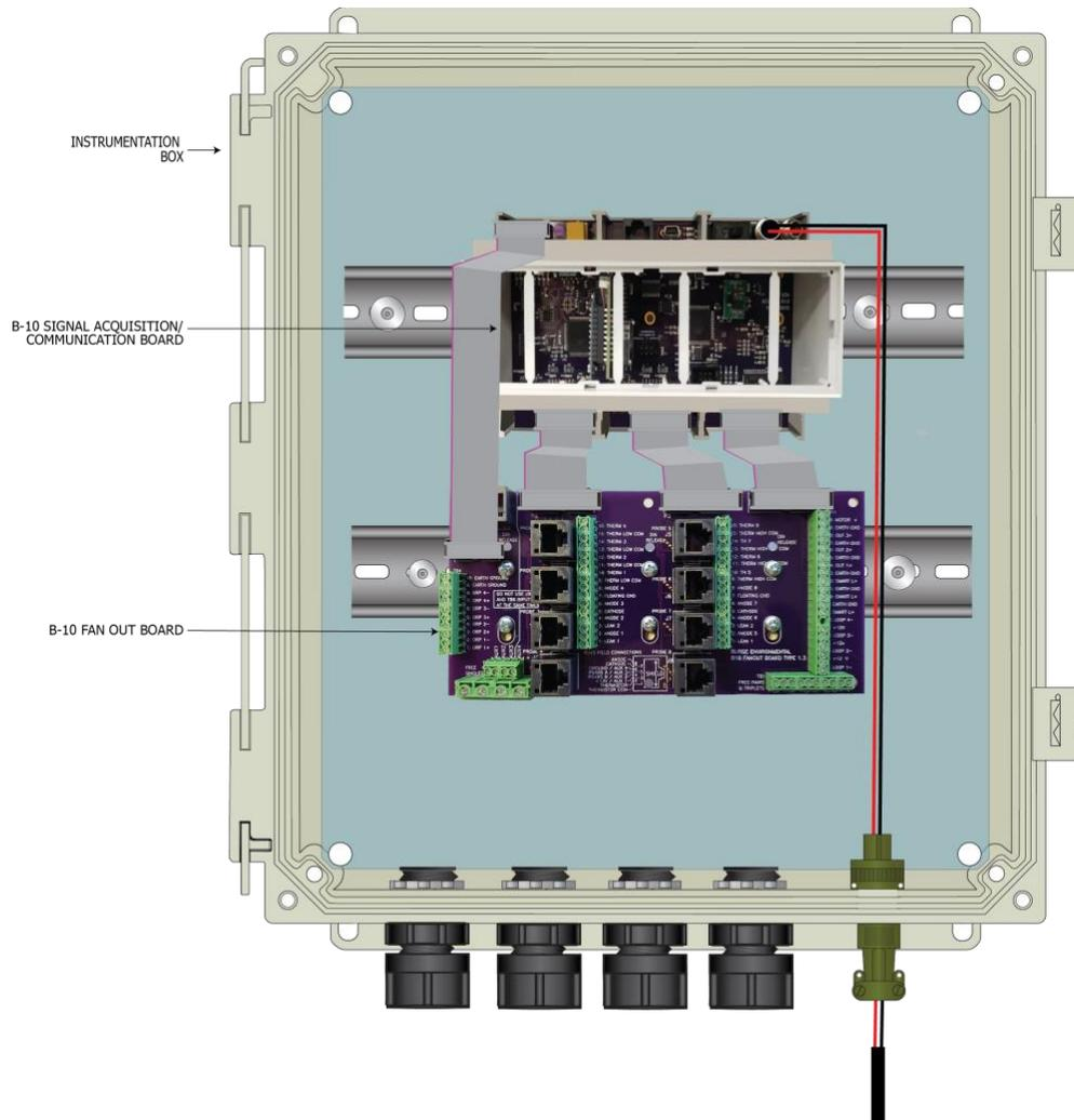
Figure 3: MiProbe Instrumentation Box, Series 200
