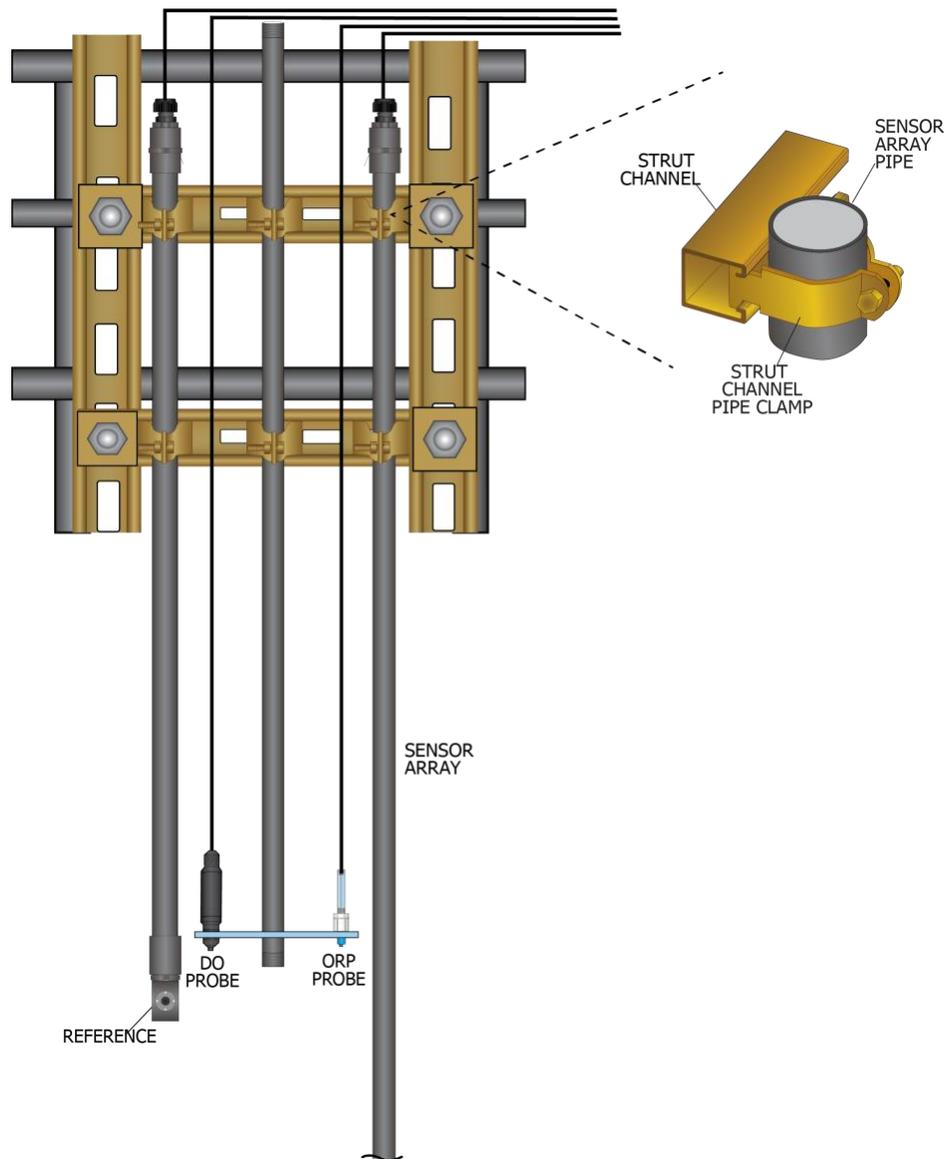
Figure 24: Mounting of the Auxiliary Sensor(s)
