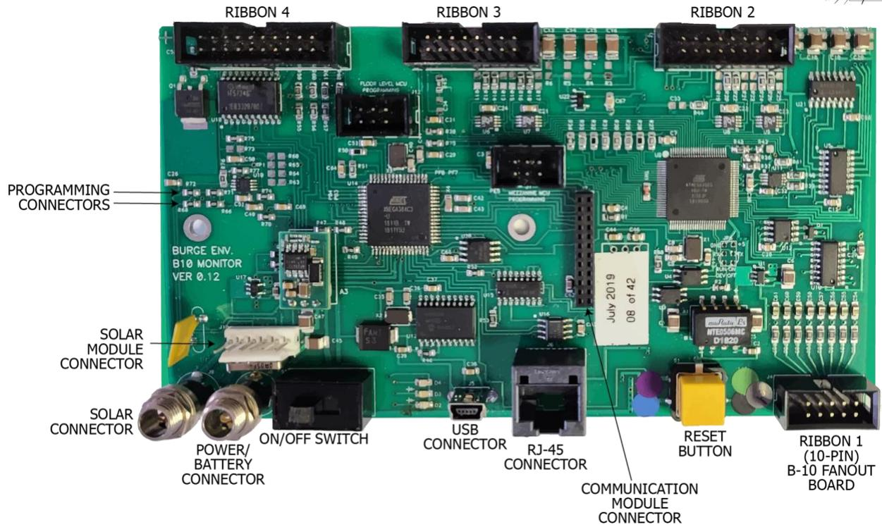
Figure 4: B10 Signal Acquisition/ Communication Board
