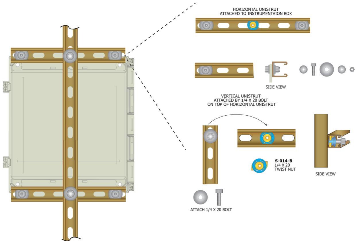
Figure 21: Mounting of the Instrumentation Box
